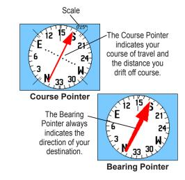
The compass ring is an electronic compass that functions like a magnetic compass when you are stationary. When you are moving and reach a pre-set speed, it uses data from the GPS receiver to maintain your heading. When you stop (after a pre-set time), it again operates like a magnetic compass. The compass ring is especially helpful when using a paper map or chart in conjunction with your GPSMAP 60CSx for navigation. When the electronic compass is on, a compass icon appears in the status bar.
