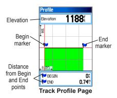
The beginning of the track is marked by a flag. You can scroll across the track profile by pressing left or right on the ROCKER.
