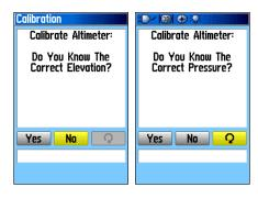
4. Use the **ROCKER** to enter the new elevation or pressure, then highlight **OK** and press **ENTER** to return to the Altimeter Page.
