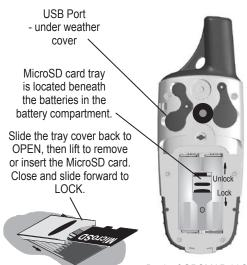
Detail of MicroSD card tray in Battery Compartment
