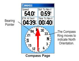
When navigating, the Compass Page provides navigation data and directions. It uses a graphic compass ring, a bearing/course pointer and digital data fields to show information such as current speed, distance to the next point on the route, estimated arrival time
